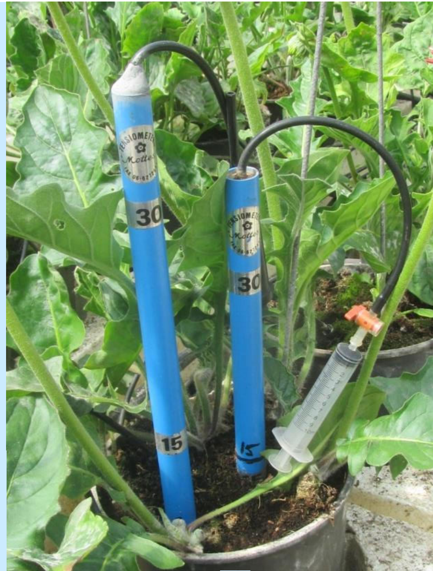
Pumping the Soil Solution.
